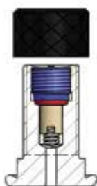
Model of valve stem integrated 7/8"14 UNF (C)
