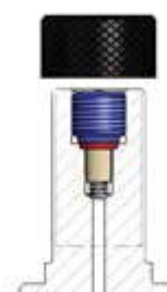
Model of valve stem integrated 5/8" 18 UNF (D)
