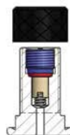
Model of valve stem integrated 7/8" 14 UNF (C)
