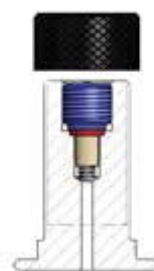
Model of valve stem integrated 5/8" 18 UNF (D)
