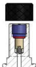
Model of valve stem integrated 7/8" 14 UNF (C)
