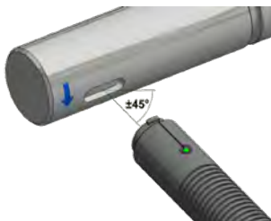
Rotating shaft: Contactless speed measurement.
