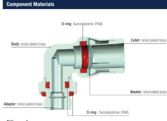
Reliable performance is dependent upon the type of fluid conveyed, component materials and tubing being used. Use is guaranteed with a vacuum of 755 mm Hg (99% vacuum).
