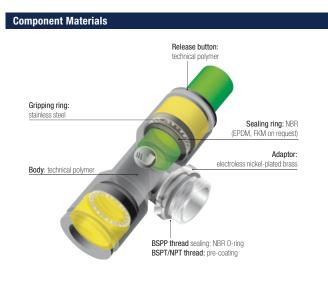
Reliable performance is dependent upon the type of fluid conveyed, component materials and tubing being used.
